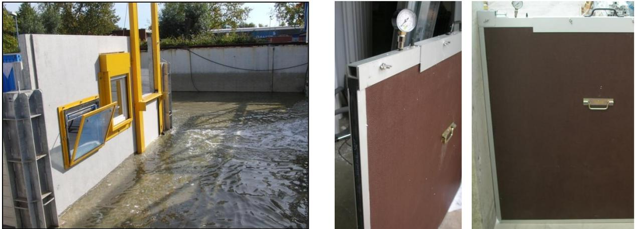
Figure 35: Aquastop system – Door, window and Figure 36: Collad'eau basement window barriers
