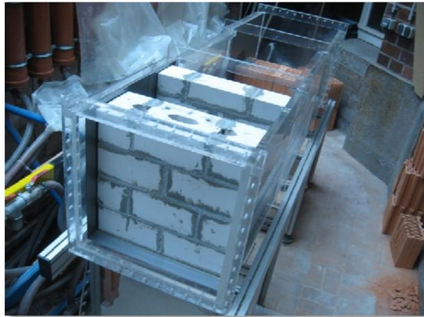
**Fig. 24: Water tank with two wall test arrangements that are under construction in-situ. In front: the double shell masonry of sand-lime bricks with heat insulation and air gap. In the background: the single shell masonry of hollow bricks with external heat insulation and ventilated curtain façade.**
