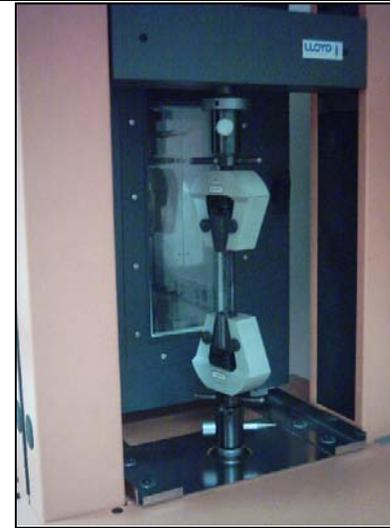
Figure 18 Lloyd Instruments. Testing facilities of mechanical properties test for rectangular specimens(3-5 mm and 20mm  $\pm$ 10%)
