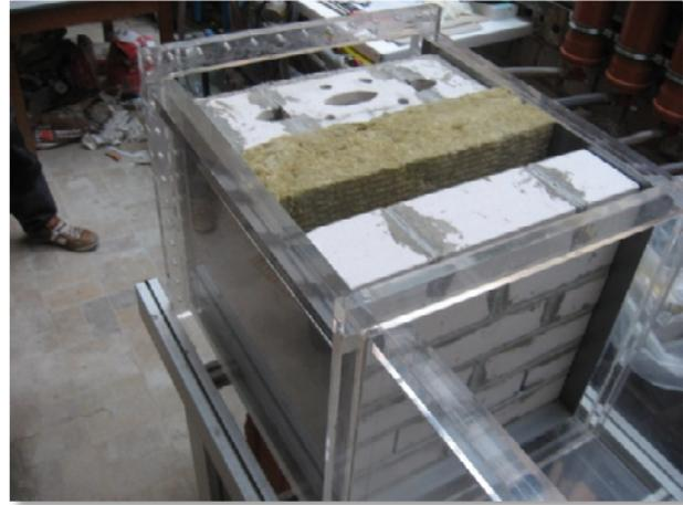
**Fig. 8: Composite wall construction; double shell masonry of sand-lime bricks with heat insulation.**
