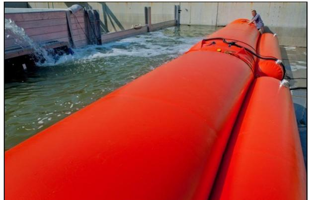
Figure 29: OPTIMAL system – water-filled double tube system
