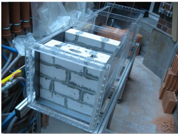
*Figure 16: Water tank with two wall test arrangements that are under construction in-situ. In front: the double shell masonry of sand-lime bricks with heat insulation and air gap. In the background: the single shell masonry of hollow bricks with external heat insulation and ventilated curtain façade.*
