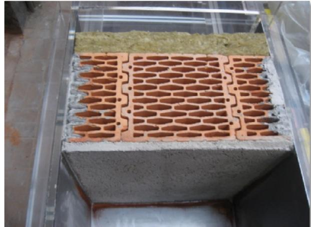
Fig. 10: Composite wall construction; single shell masonry of hollow bricks with external heat insulation and ventilated curtain wall; the curtain façade board is not yet mounted here.
