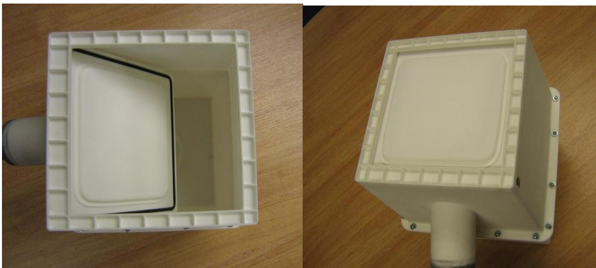
Figure 39: Non-return valve, in open and closed positions.
