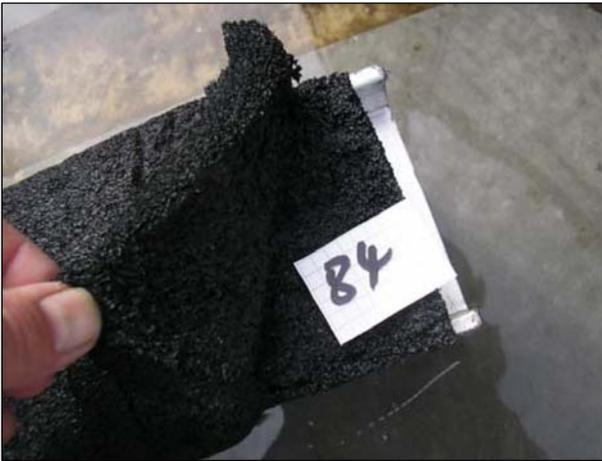
Fig. 9: Cracked ground seal at the end of the destructive testing<sup>36</sup>
