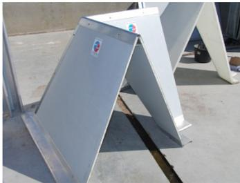
Hexagonal Aluminium comb panel „ALUCORE 15“ + Aluminium coating
