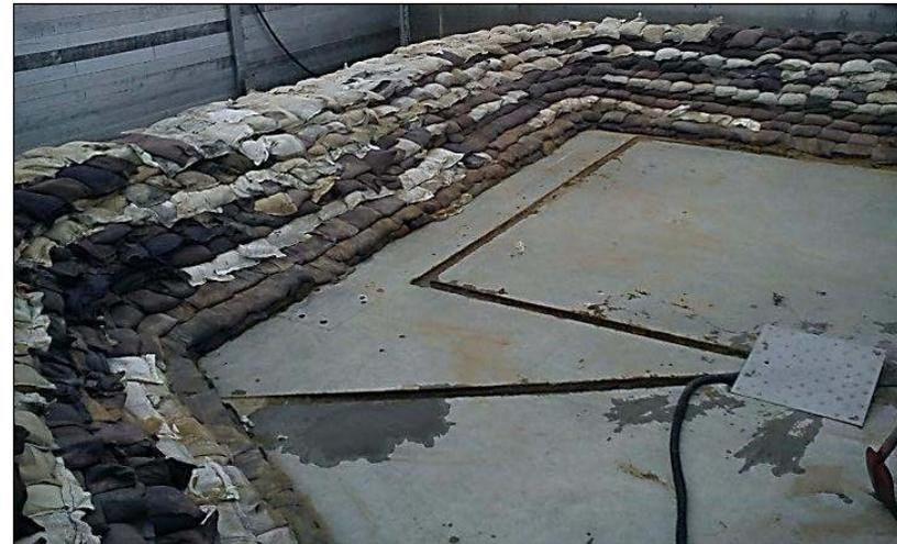
Fig. 6: Filled sandbags on pallets and built sandbag dam according to FM Approval in the testing facility of the TUHH in Hamburg-Wilhelmsburg<sup>22</sup>
