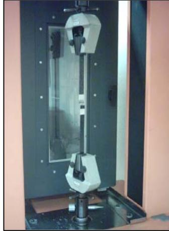
Figure 17 Lloyd Instruments . Test facility of adhesion test for rectangular specimens(wide:25mm  $\pm$  5% and long: 100mm $\pm$ 5%)
