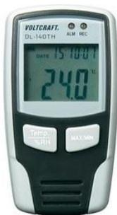
*Figure 14: Digital data-logger to record air temperature and relative humidity in the laboratory at regular intervals.
