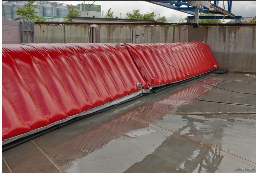
Fig. 6: Straight product configuration of the system DADLER in the testing facility of the TUHH in Hamburg-Wilhelmsburg<sup>13</sup>
