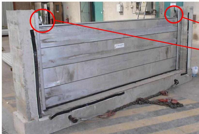
Figure 1 : Barrier n°4 elements stacked between columns
