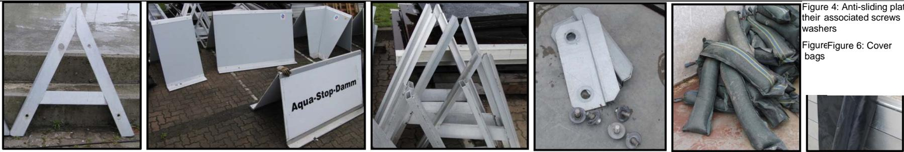
Figure 4: Anti-sliding plates with their associated screws and washers
