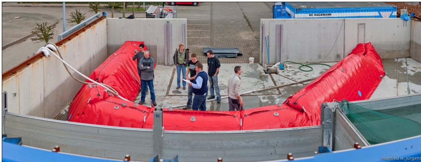
Fig. 5: Product configuration of the system DAEDLER according to FM Approval in the testing facility of the TUHH in Hamburg-Wilhelmsburg<sup>12</sup>
