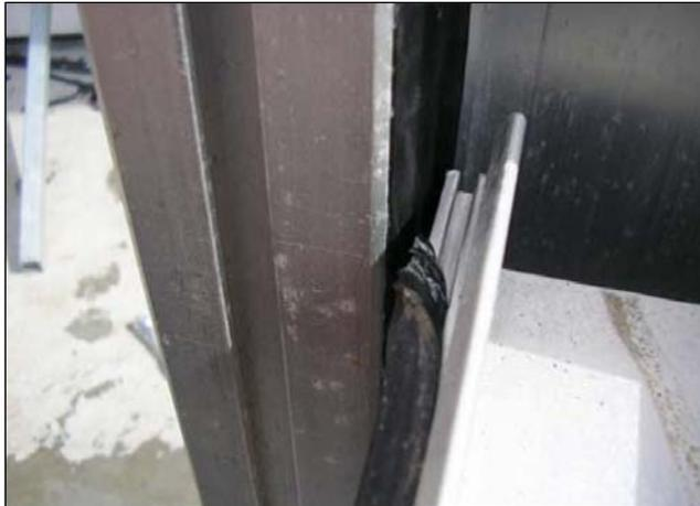
Fig. 7: Loose seals at the end of the destructive testing<sup>36</sup>
