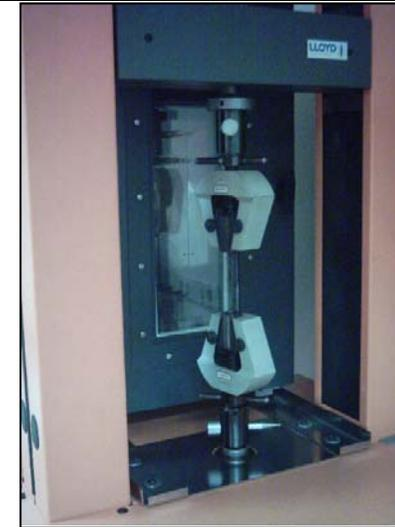
Figure 2 Lloyd Instruments. Testing facilities of mechanical properties test for rectangular specimens(3-5 mm and 20mm  $\pm$ 10%)
