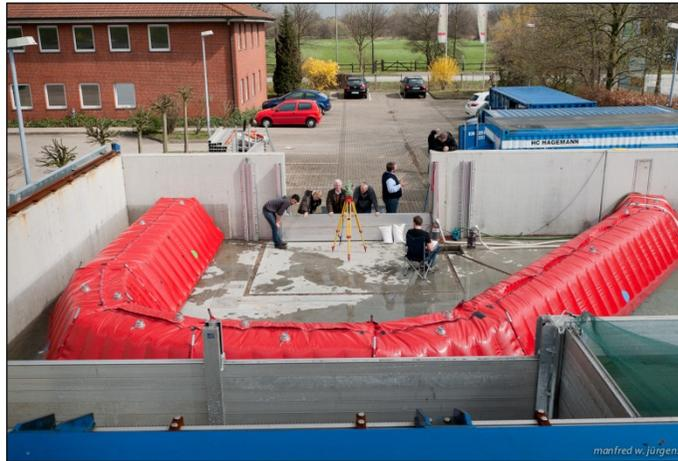
Fig. 1: Trapezoidal tube flood protection system DAEDLER in the testing facility of the TUHH in April 2011<sup>7</sup>
