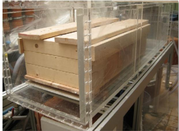
**Fig. 16: Suspended timber floor; test arrangement consisting of structural joists, heat and sound insulation, plasterboard ceiling, and covering floor boards**
