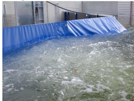
Figure 5 :Hydrodynamic load / current load executed perpendicular to the barriers
