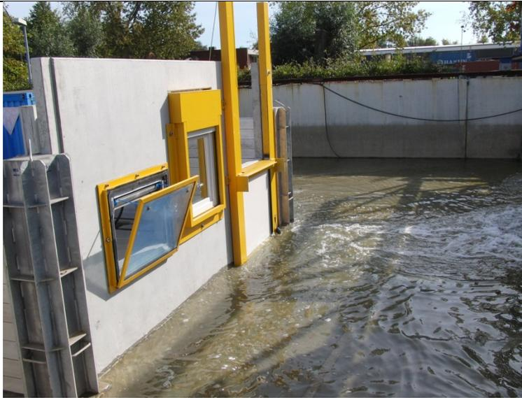
Fig. 1: Door, window and basement window barriers
