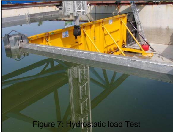
Figure 7: Hydrostatic load Test
