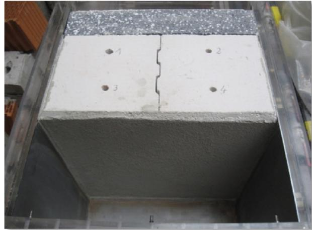
**Fig. 14: Composite wall construction; single shell wall of light (aerated) concrete blocks with thermal insulation composite system.**
