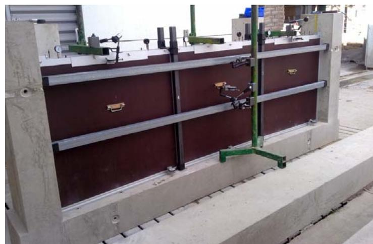
Figure 2 : Hydrostatic test on flood barrier Collad'eau (width 3m)
