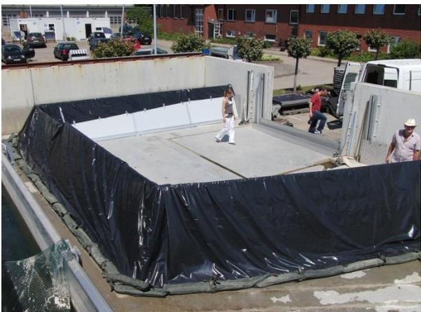
Figure 30: AQUASTOP Damm – demountable perimeter flood barrier
