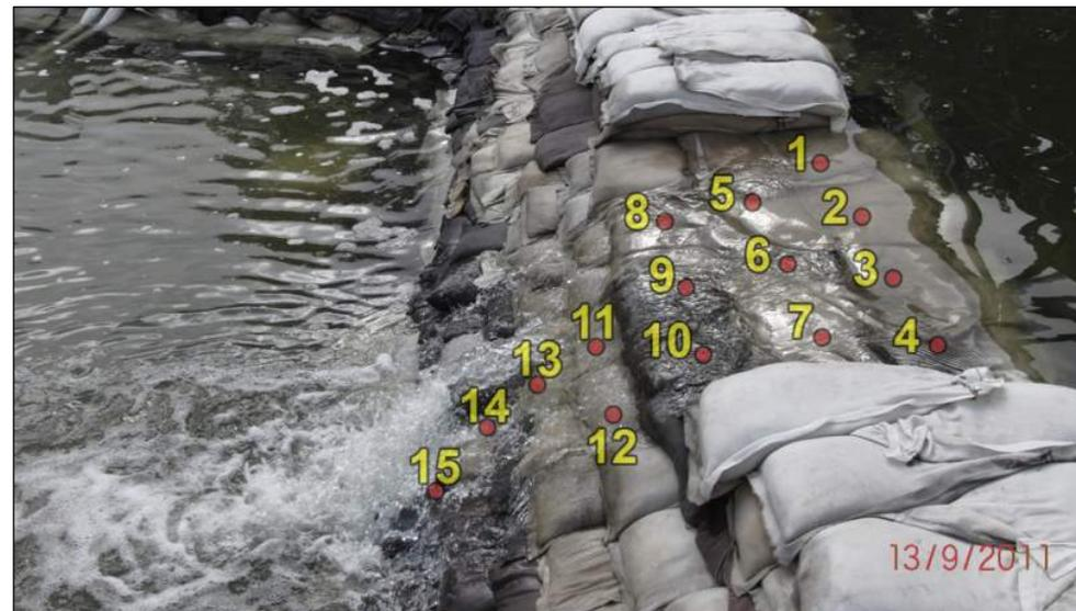
Fig. 8: Overflow test in the testing facility of the TUHH in Hamburg-Wilhelmsburg<sup>22</sup>
