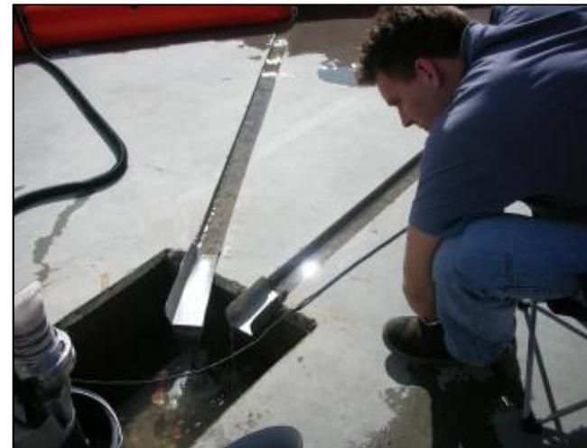
Fig. 4: Pump sump for leakage measurement<sup>3 oben3</sup>
