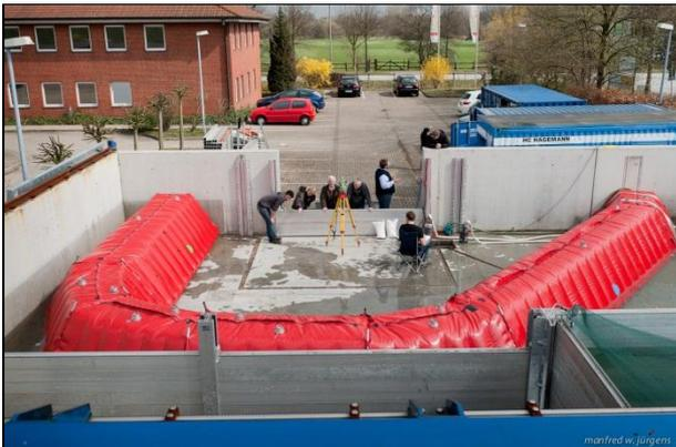
Figure 28: DAEDLER system – trapezoidal water-filled tube system
