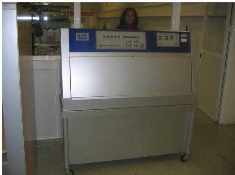
*Figure 24: Resistance to UV radiation in presence of moisture. Ref: Sika*
