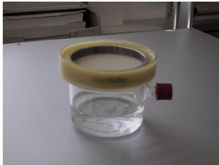
Figure 7: Water vapor permeability
