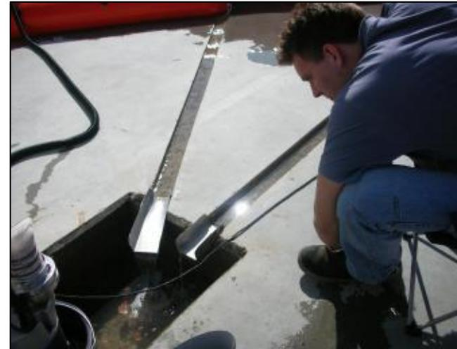
Fig. 3: Pump sump for leakage measurement<sup>3 oben3</sup>
