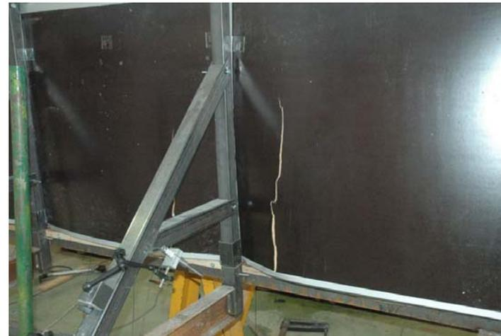
Figure 15 : rupture of the barrier
