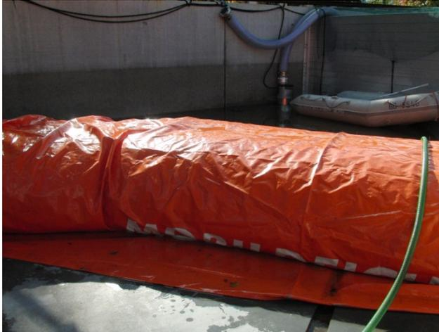
Fig. 1: Mobildeich MD93-2 installed at the water basin of the TUHH
