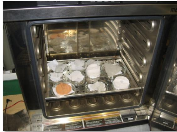
Fig. 26: Building material test samples in the drying oven to determine their oven-dry mass.
